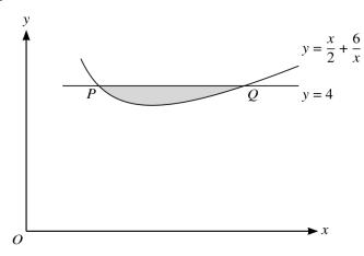
The diagram shows part of the curve  $y = \frac{x}{2} + \frac{6}{x}$ . The line y = 4 intersects the curve at the points P and Q.
