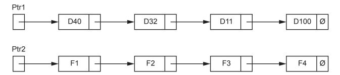
(a) The linked list is implemented using two variables and two 1D arrays as shown.
