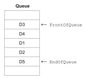
The queue is implemented using three variables and a 1D array of eight elements as shown. The variable <code>NumItems</code> stores the number of items in the queue.
