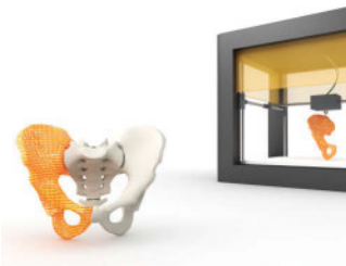
▲ Figure 3.12 Artificial bone framework made using an industrial 3D printer
